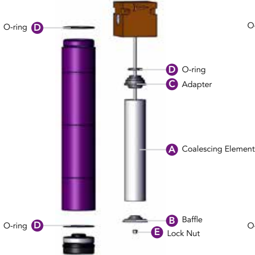
Figure 2 : Oil Coalescing Filter
